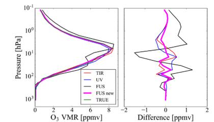
Figure 7. The fused profile and the residual error obtained with the modified algorithm (magenta lines) compared with the same quantities of Fig. 3b and c.
